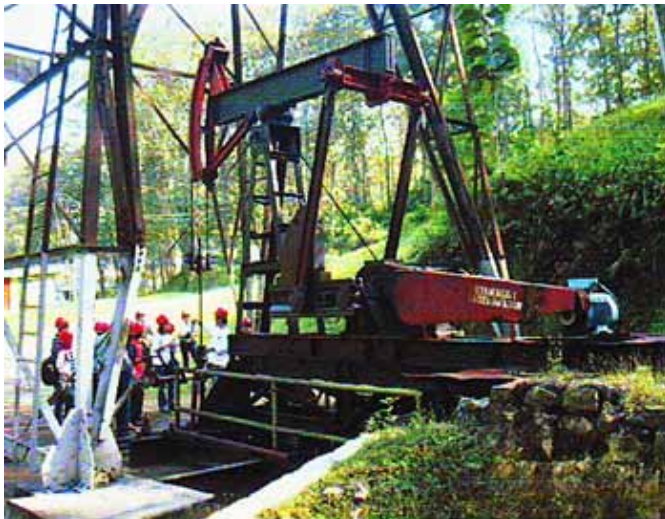
Figure 3. Beam Pump at Ledok Field. Old Pumping Unit "THOMASON" BPM (1894) at Ledok Field. Still actively operating, with Ngrayong Sand reservoir at 1000 m deep.
