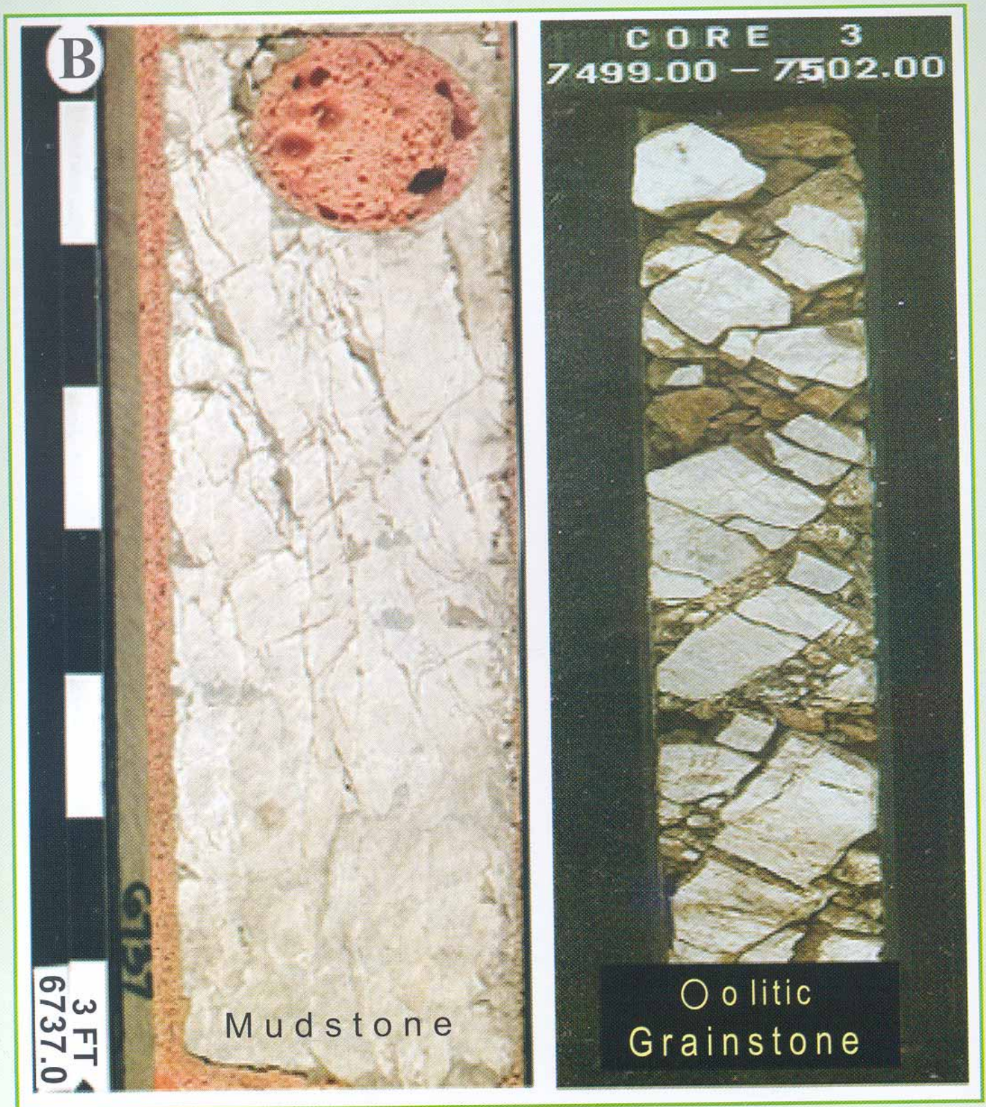
Figure 4: An example of fracturing in the fine- grained (mud matrix supported) facies and coarse- grained (grain supported) facies. The larger scale fractures are better developed in the coarse-grained facies of the Manusela Formation
